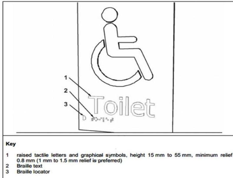
**Figure 88: Details of raised tactile sign dan Braille**
