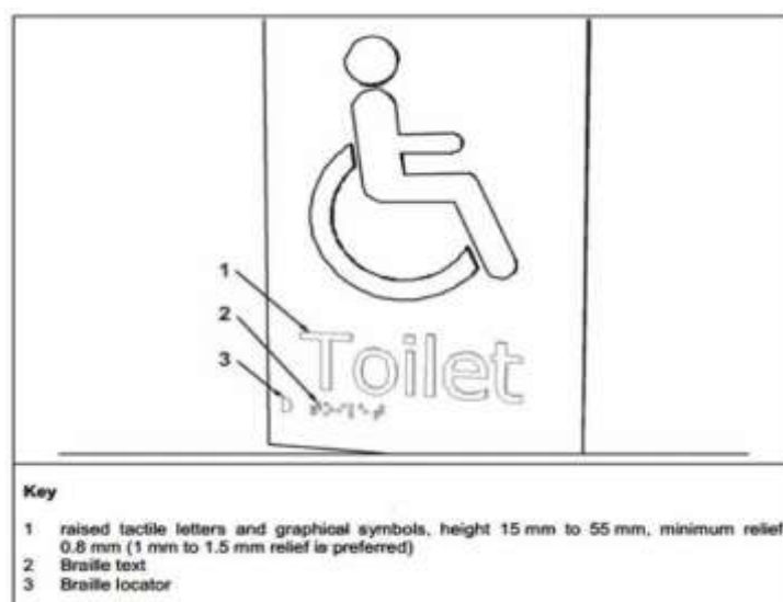
Figure 88: Details of raised tactile sign dan Braille
